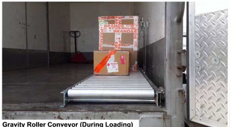
Gravity Roller Conveyor (During Loading)
