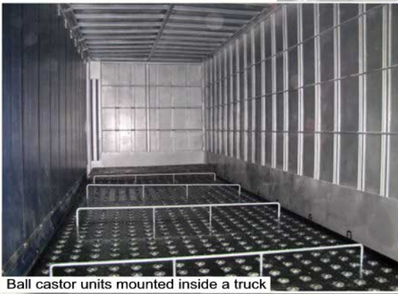
Ball castor units mounted inside a truck
